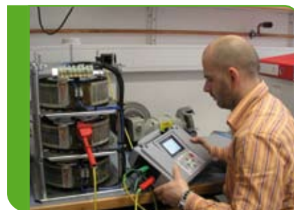
Shielded test leads 10 kV included in standard set
